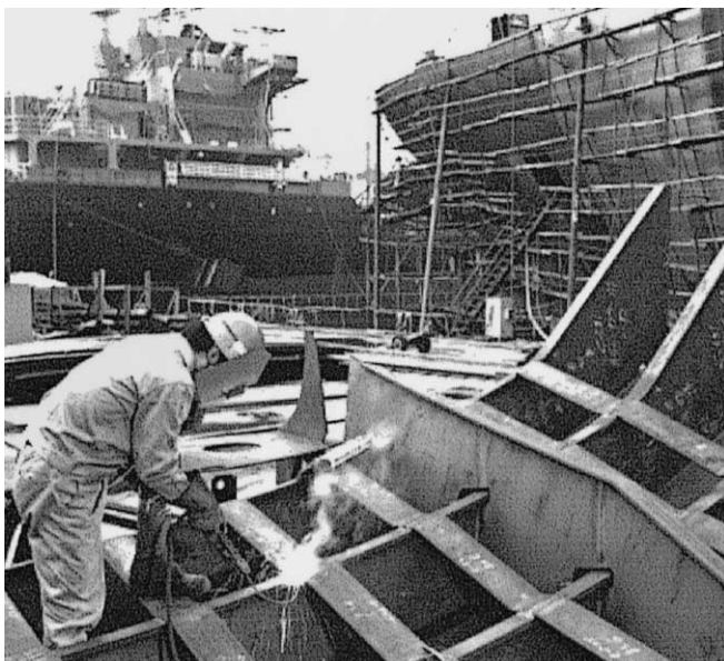
Fig. 1 - Ilmenite type electrodes shined in shipbuilding throughout the 1960s and 1970s due to excellent usability and weldability
